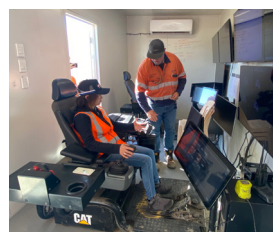
Remote control of mining equipment
