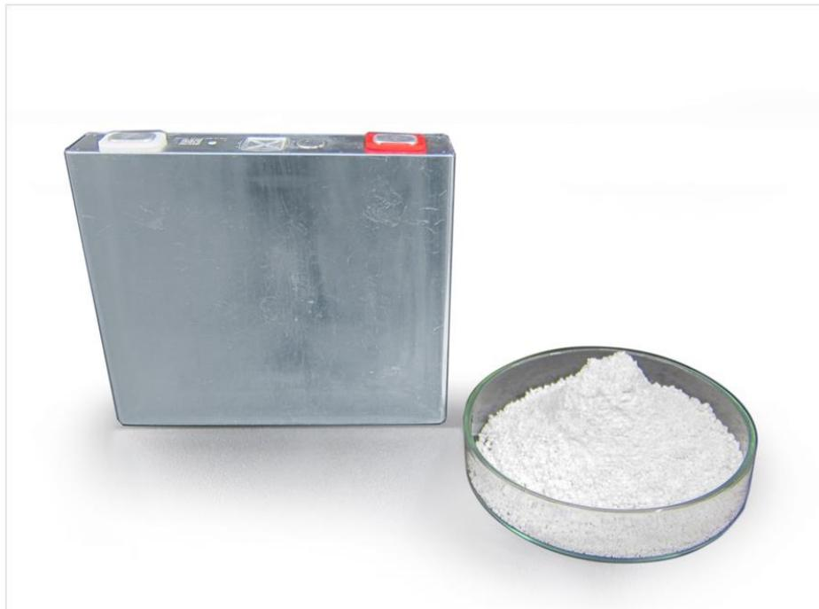
Prototype cell & Niobium Titanium Oxide (NTO)
