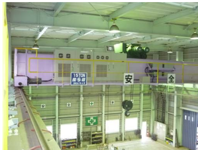
A hybrid crane equipped with a lithium-ion capacitor
