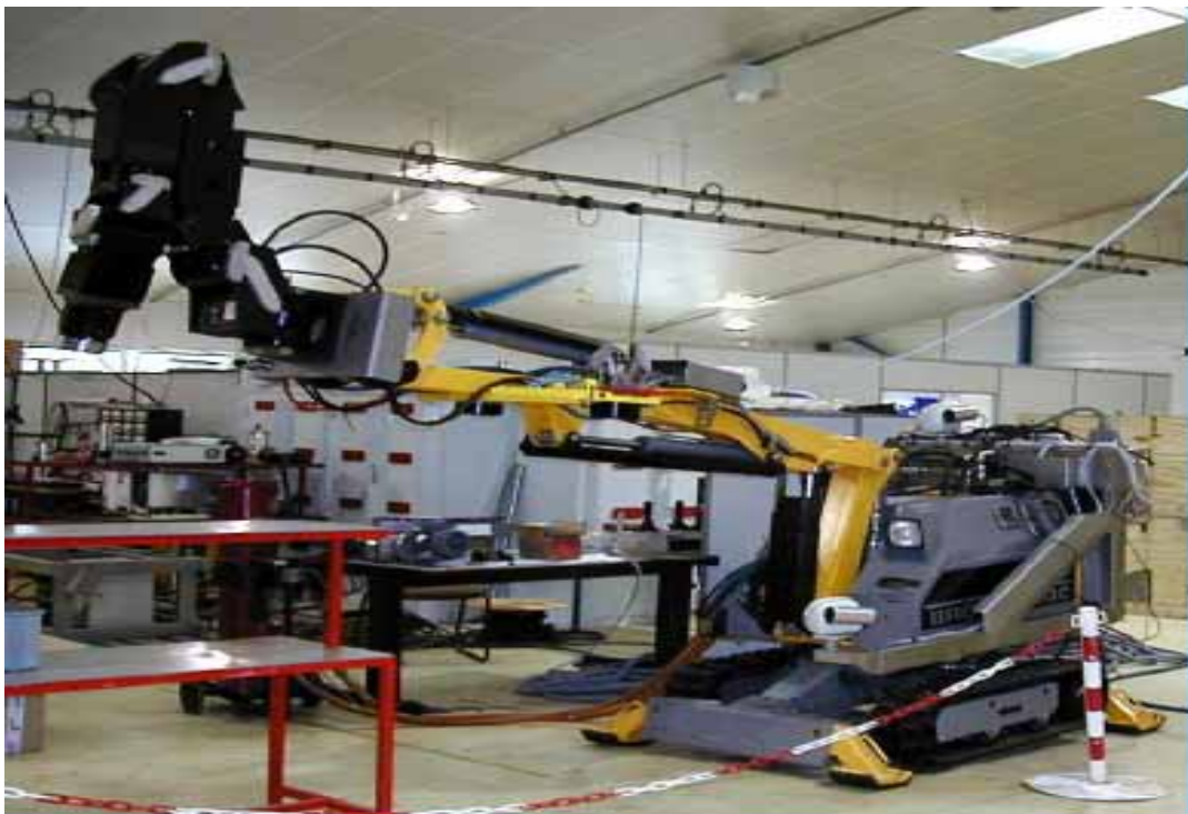
Remote-controlled small bulldozer mounted arm system (one of the examples)
