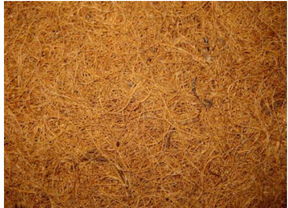
4) Coconut fiber pressed into sheets
