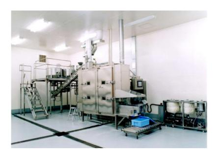
The rice cooking system has three inner layers. Each layer has a stainless steel mesh belt conveyor, onto which rice is placed before being sequentially fed to the upper, middle and the bottom layers. The upper (80 - 100°C) and middle (120 - 140°C) layers are used for the boiling and steaming process, during which the system agitates the rice as it sprays hot water to complete steaming. The bottom layer is
